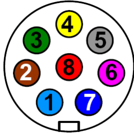
Figure 4: Front panel jack pin assignment, front view of the 8 pin Binder 712 female connector
